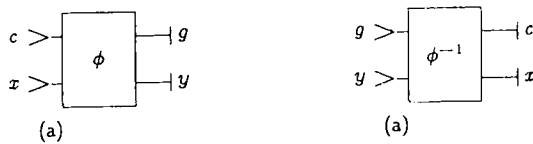
Fig. 20. (a) Computation of y = f(x) by means of a combinational conservative-logic network \phi . (b) This computation is “undone” by the inverse network, \phi^{-1} .
